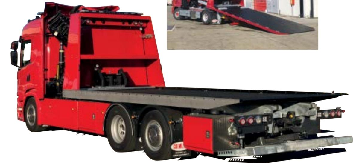
The Equipment **ST 400** is unstoppable, with its superstructure it is able to load vehicles with heavy weights without the minimum effort. The double steel guides make it possible to carry out work that is risky for other installations. This structure can mount 4 or 6 Ton forks for the rescue of heavy vehicles. Available in the version with aluminum alloy platform "AL400" is applicable on vehicles from 18 to 32 tons.
