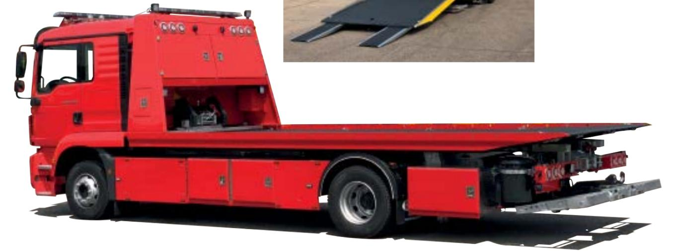
The Equipment **SE 200** is fast and reliable, suitable for the recovery and transport of all types of vehicles. Its double movement allows to better manage the loading and unloading of cars. Available in the version with aluminum alloy platform "SEA200" is applicable on vehicles from 7.5 to 18 tons.
