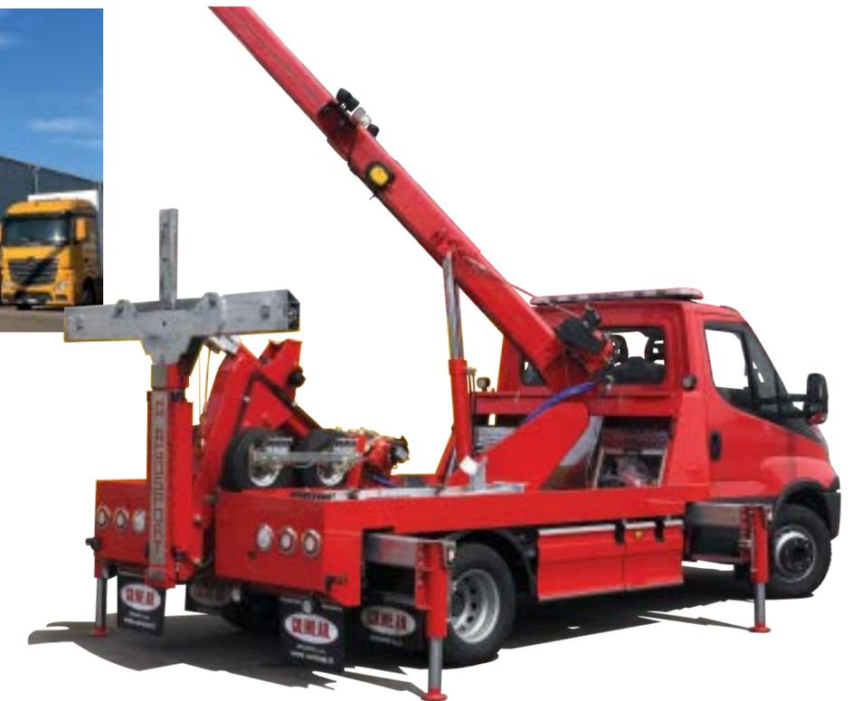
The equipment **RFTG** represents the optimal solution for the removal of vehicles, thanks to its revolving crane boom with double hydraulic extension. Available with rear fork with automatic opening and closing (RFTG 020) it is famous for its extreme ease and speed of intervention in any situation, able to remove a car parked or broken in a minimum amount of time. Applicable on vehicles with total mass from 5 to 10 tons.
