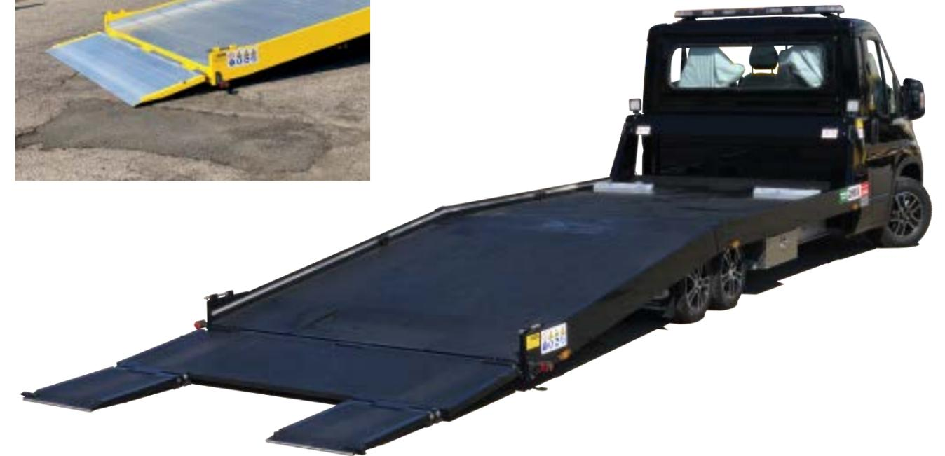
The Equipment **PF 1500** is perfect for transporting vehicles, equipped with a completely aluminum alloy frame and a homologated double rear axle allowing a payload of 1200 kg. The reduced height from the ground and the lowerable axles allow to reduce the inclination and to be able to easily load cars with sports suspension and supercar. Applicable on chassis with a total mass of 3,5 Ton.
