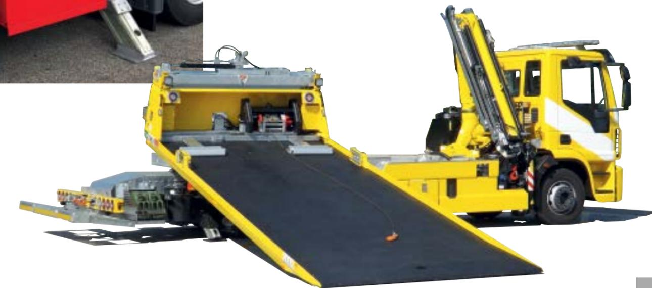
The Equipment **SEA 200G** is unique in its kind and innovative for vehicle recovery. Equipped with a platform that rotates 180° through a hydraulic gearmotor, it can recover vehicles with extreme ease in situations of reduced maneuvering space, facilitating recovery beyond ditches, guardrails or unevenness. Available in the version with hot-galvanized steel platform "SE200G" it can be applied on vehicles from 12 to 18 tons.
