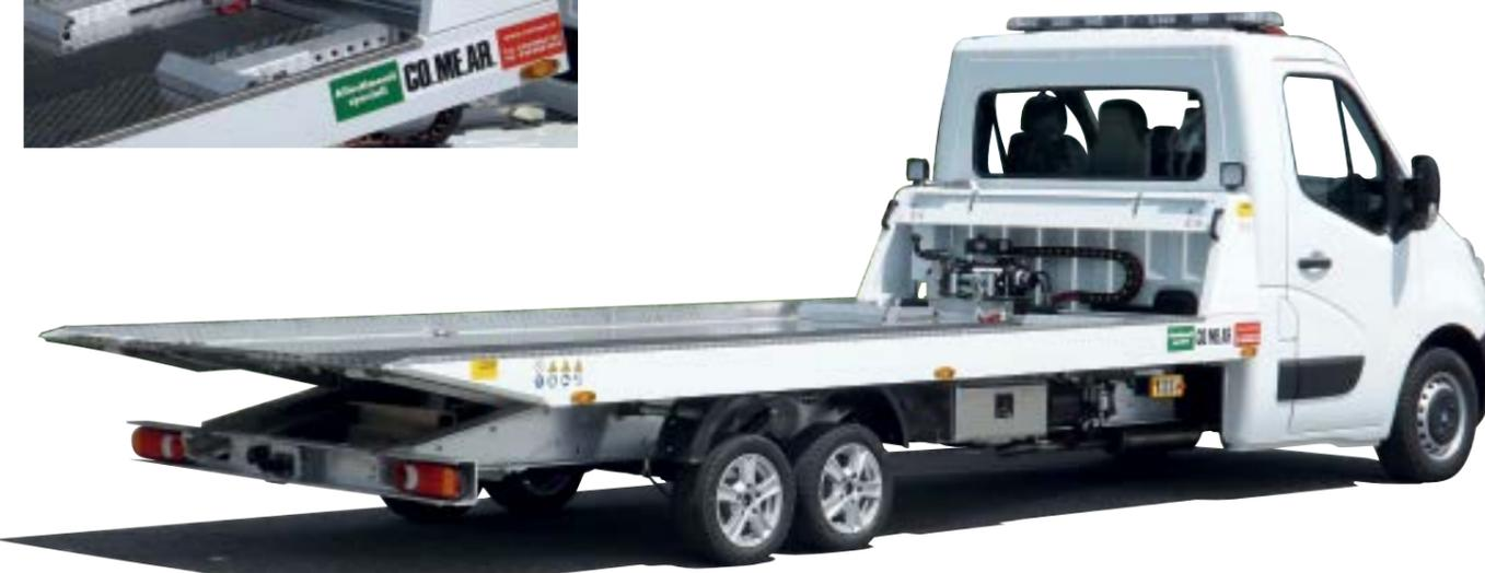
The Equipment **SP 1250** is a hybrid between CITY STAR and PF1500, equipped with a frame completely in aluminum alloy, with a homologated double rear axle allowing a payload of 1100 kg. Thanks to the sliding platform it is suitable for roadside assistance, at the same time excellent for loading cars with sports suspension. Applicable on chassis with a total mass of 3,5 Ton.
